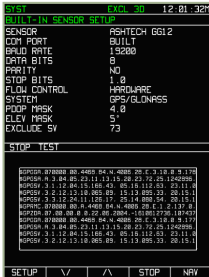
7-101: SYST page during testing of the GNSS sensor and its communication channel
