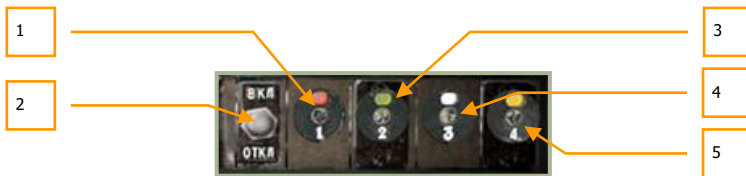
6-49: Signal flare control panel
