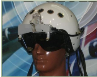
14-8: Helmet Mounted Sight (HMS) targeting system
