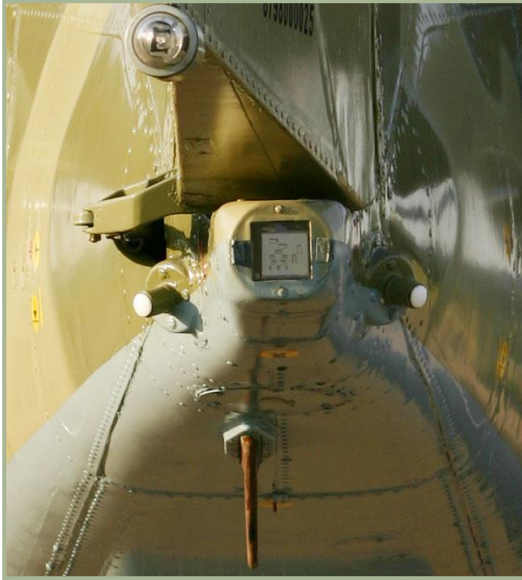
1-6: The tail of the Ka-50. The white navigation light is located at the top of the image. The L-140 laser sensor system is in the center and various IFF antennas are located on each side and below.
