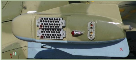
1-8: UV-26 flares dispenser, left (red) navigation light and the signal flare
