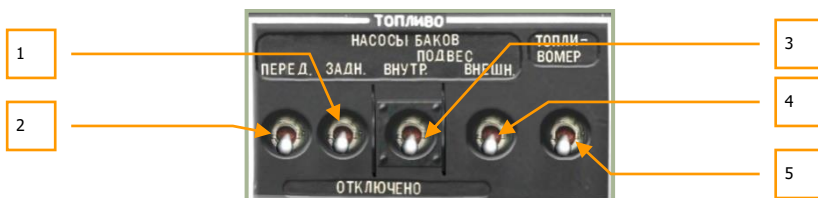
6-54: Fuel pump controls
