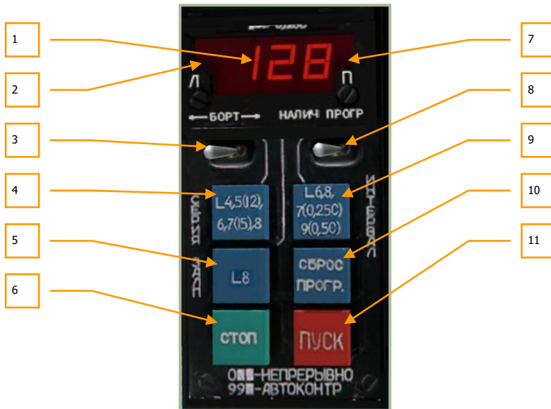
6-34: UV-26 Countermeasures control panel
