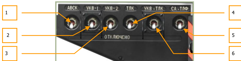
6-53: Radio and data link power control panel
