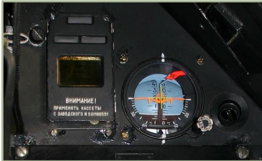
1-5: Ekran built-in warning and control system (left) and auxiliary flight indicator
