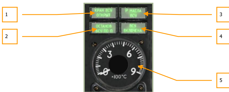
6-78: Auxiliary Power Unit (APU) panel
