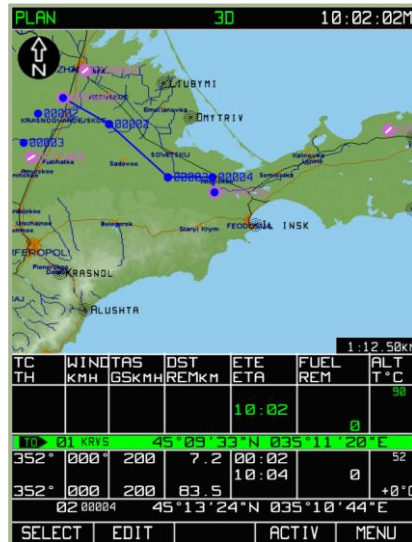
7-73: Result of inverting route
