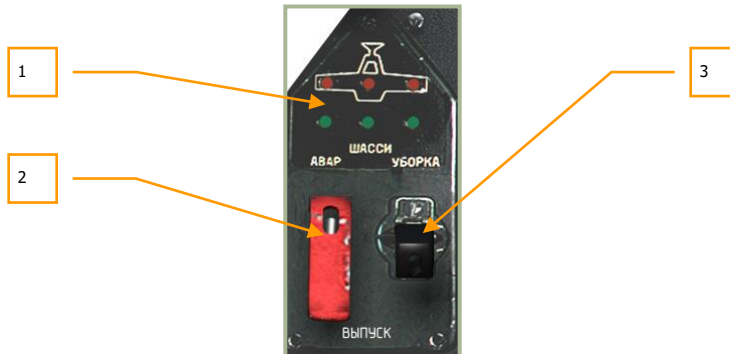
6-29: Gear control panel
