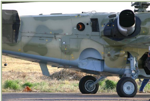
1-3: The exhaust nozzle of auxiliary power unit (in operate) and screen-type exhaust
