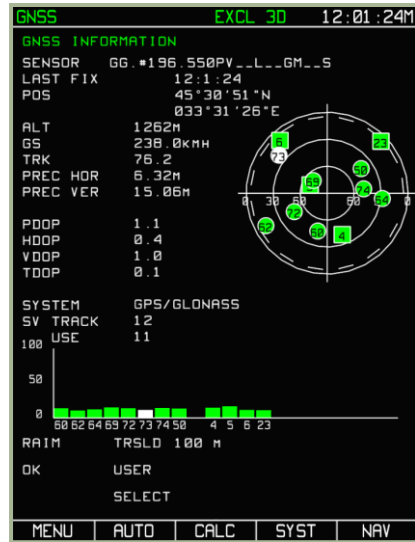
7-101: SYST page during testing of the GNSS sensor and its communication channel
