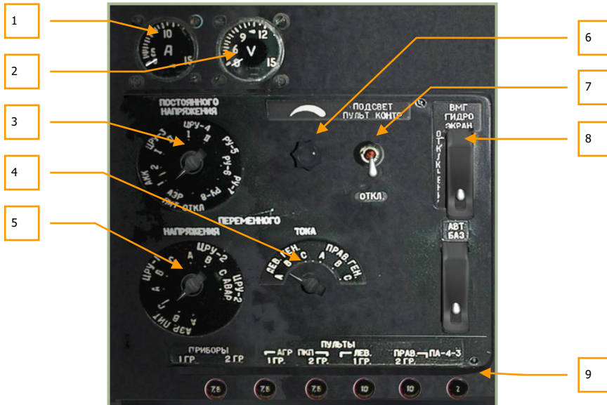
6-71: Electrical System Control panel
