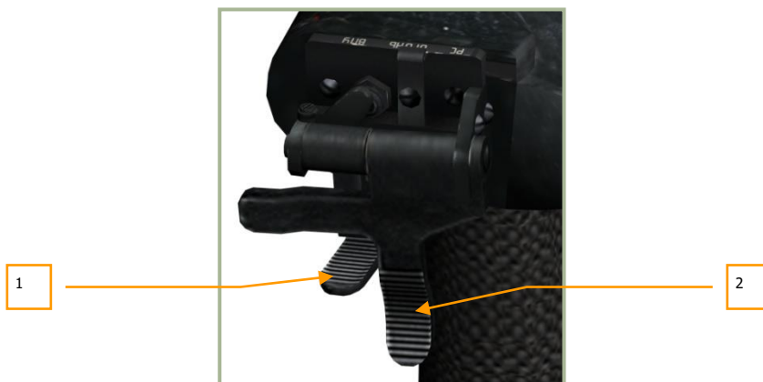
6-6: Weapon (large) and Cannon (small) triggers in default position – Release Weapon trigger operates
